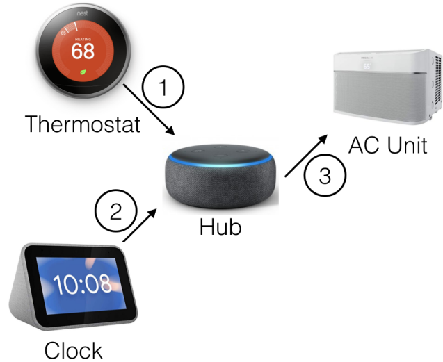
Figure 3: Control flow of a thermostat and a clock turning on the air conditioning unit. In (1), the thermostat sends a temperature update to OrbanHub. Then, in (2), the clock sends its update to OrbanHub. Finally, in (3), OrbanHub constructs a proof along with the command to the air conditioning unit.
